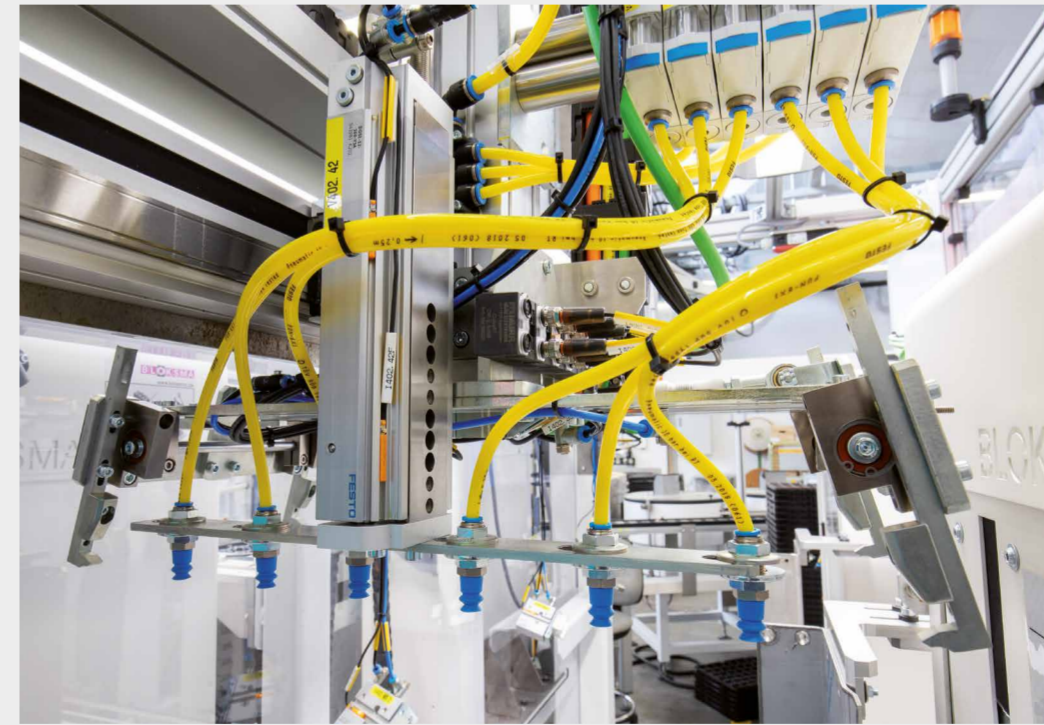
The modules are mounted right next to the sensors and actuators – at the heart of the process – for example on pneumatic devices or grippers.
