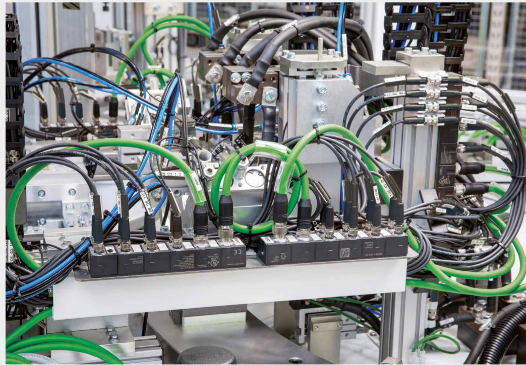
Hager engineers can decide whether they want to use each port as an input or output – this turn standard modules into customized modules.
